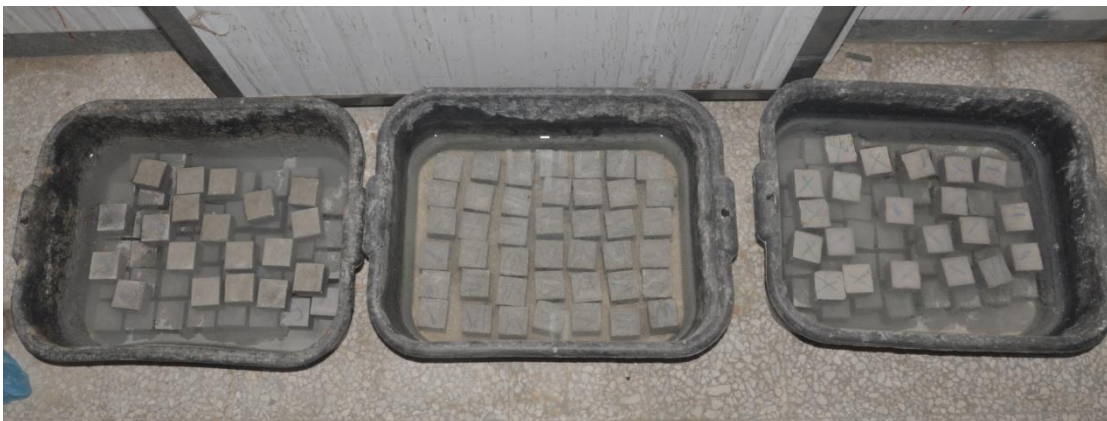
Figure 3.6: Curing of specimens in water tanks.
